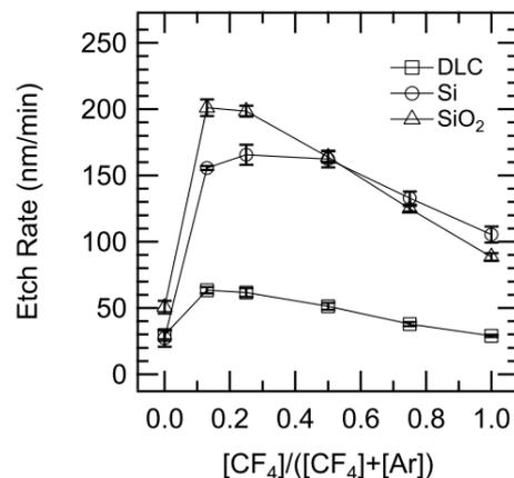
**Figure 1** – Etch rate of the DLC in the  $\text{CF}_4/\text{Ar}$  plasmas plotted with those of Si and  $\text{SiO}_2$  as a function of the gas-mixture ratio of  $[\text{CF}_4]/([\text{CF}_4]+[\text{Ar}])$ . The self-bias voltage was constant at -100 V. Error bars indicate variability in reproducing the experiments of etching and measuring the steps on the samples by stylus profilometry
