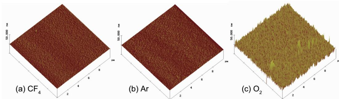
**Figure 5** – AFM images on surfaces of the DLC samples etched in the (a) pure-CF<sub>4</sub>, (b) Ar and (c) O<sub>2</sub> plasmas. The RMSs indicating roughness on the surfaces in the pure-CF<sub>4</sub>, Ar and O<sub>2</sub> plasmas were 0.084, 0.094 and 1.7 nm, respectively
