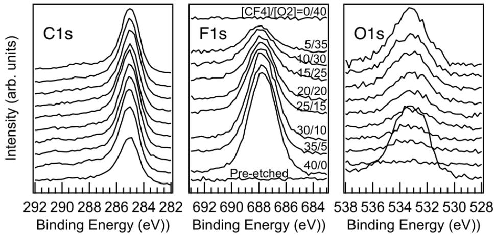
**Figure 4** – XPS spectra of C<sub>1s</sub>, F<sub>1s</sub> and O<sub>1s</sub> on surfaces of the DLC samples etched in the CF<sub>4</sub>/O<sub>2</sub> plasmas, and on that of a pre-etched one. The experimental conditions were the same as in Figure 3
