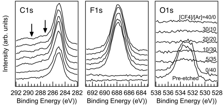
**Figure 2** – XPS spectra of  $\text{C}_{1s}$ ,  $\text{F}_{1s}$  and  $\text{O}_{1s}$  on surfaces of the DLC samples etched in the  $\text{CF}_4/\text{Ar}$  plasmas, and on that of a pre-etched one. The experimental conditions were the same as in Figure 1. Arrows show signals from chemical bond components of C– $\text{CF}_x$  at 287.3 and CF at 289.5 eV
