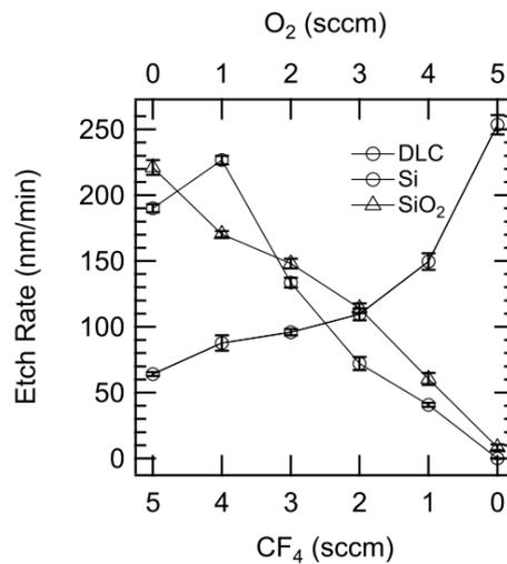
**Figure 6** – Etch rate of the DLC in the CF<sub>4</sub>/O<sub>2</sub>/Ar plasmas plotted with those of Si and SiO<sub>2</sub> as a function of the gas flow rates of CF<sub>4</sub> or O<sub>2</sub>. Etching was performed in changing gas-mixture ratio of [CF<sub>4</sub>]/[O<sub>2</sub>] with Ar dilution of 30 sccm. The total flow rate was constant at 40 sccm. The error bars are treated as in Figure 1
