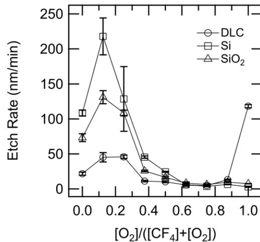
**Figure 3** – Etch rate of the DLC in the  $\text{CF}_4/\text{O}_2$  plasmas plotted with those of Si and  $\text{SiO}_2$  as a function of the gas-mixture ratio of  $[\text{O}_2]/([\text{CF}_4]+[\text{O}_2])$ . The self-bias voltage was constant at 100V. The error bars are treated as in Figure 1
