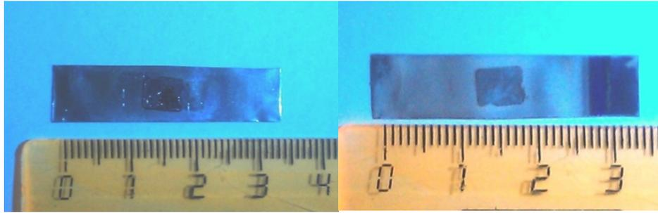
Figure 3 – Nickel foil before and after diffusion
