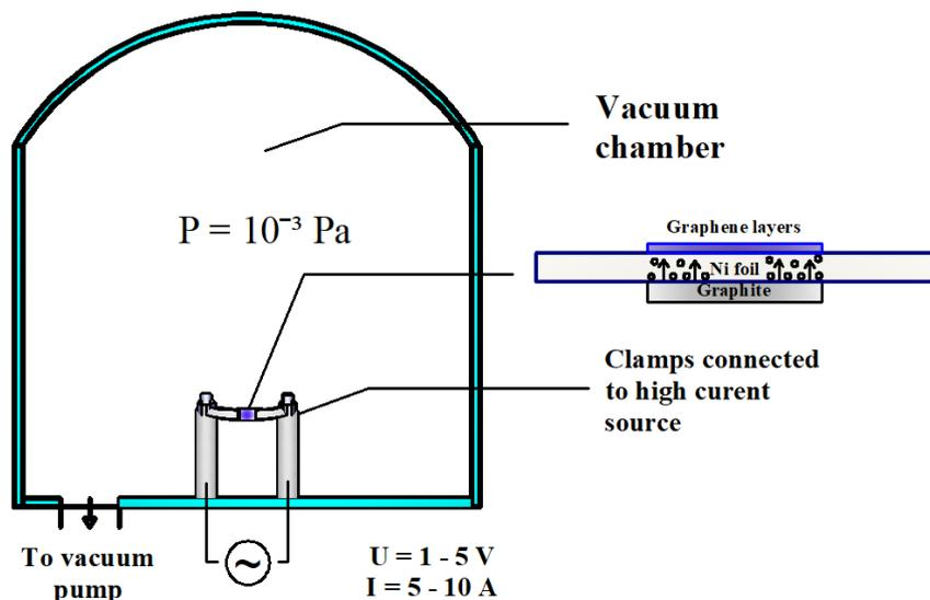
Figure 1 – Experimental setup of graphene production method
