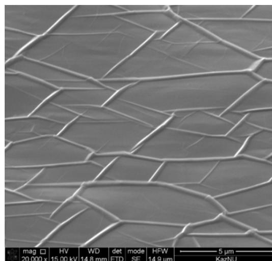
Figure 2 – SEM image of graphite layers
