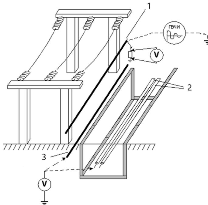
**Figure 7** – Scheme for simulating radiated impulse noise.
