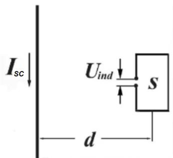
Figure 2 -  $I_{sc}$  - short-circuit current,  $U_{ind}$  - induced voltage,  $S$ -area of the circuit of relay protection and automation,  $d$ - distance from the overhead line (busbar) to the cable channel
