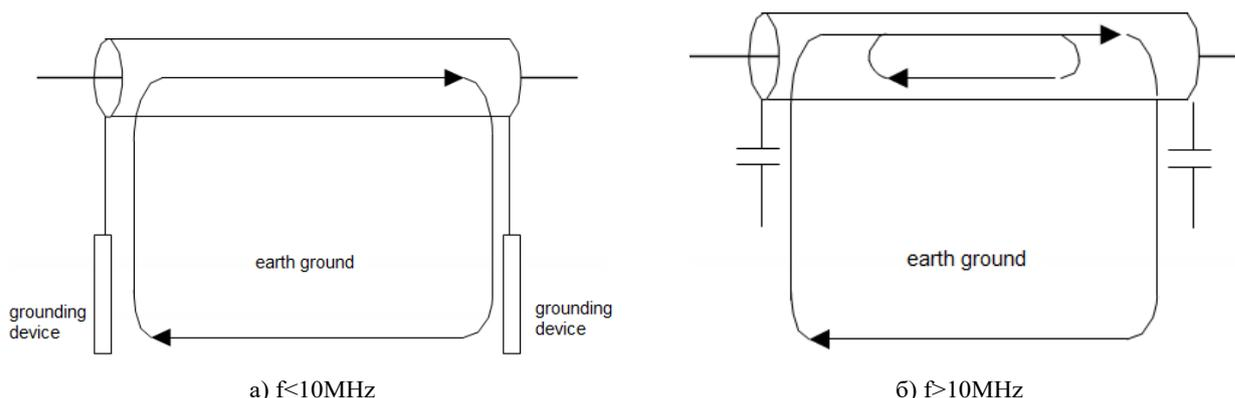
Figure 6 – Shielding current paths depending on the frequency of the interference
