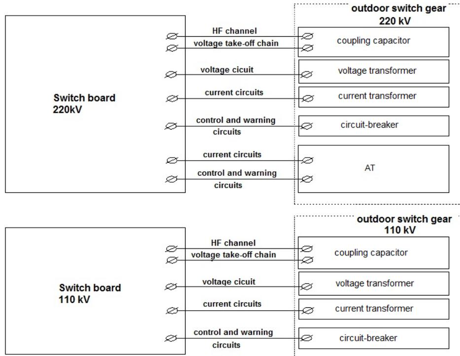
Figure 1 - Connection of relay protection and automation equipment with high-voltage equipment SS-220kV "Karatau"
