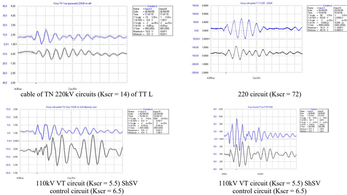
Figure 8 – Results of measuring the screening coefficient
