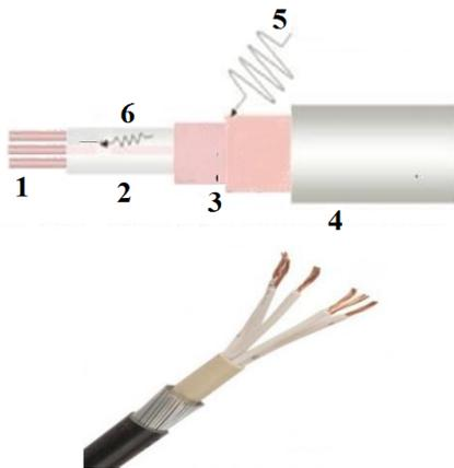
**Figure 3** - ASTU cable: 1-cores, 2-insulation, 3-shield, 4-sheath, 5-external interference (SMI), 6-residual interference (RI).
