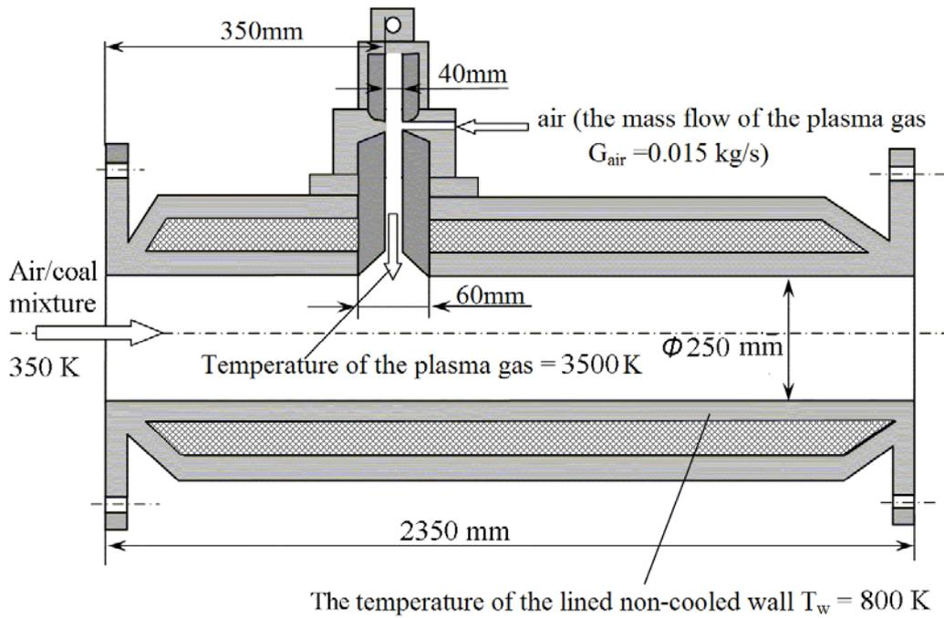
Figure 3 – Diagram of the full-scale muffle.
