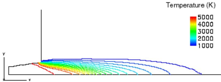
**Figure 7** – Predicted isotherms of air-plasma flow from the plasmatron (temperature, K).
