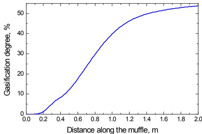
**Figure 6** – Gasification degree variation along the muffle
