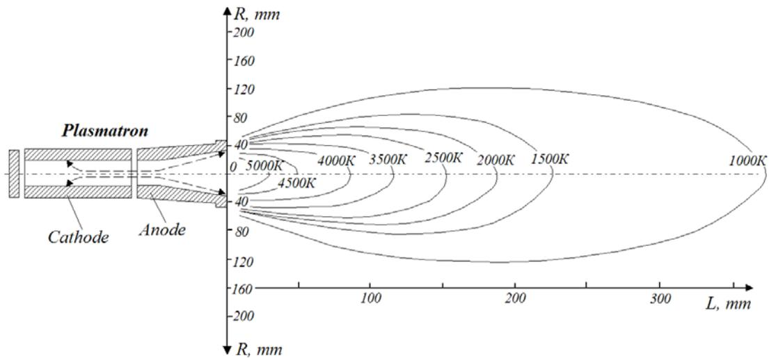
**Figure 2** – Isotherms of the air-plasma flow from a plasmatron
