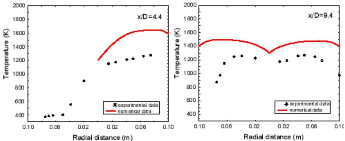
Figure 8 – Predicted radial temperature profiles.
