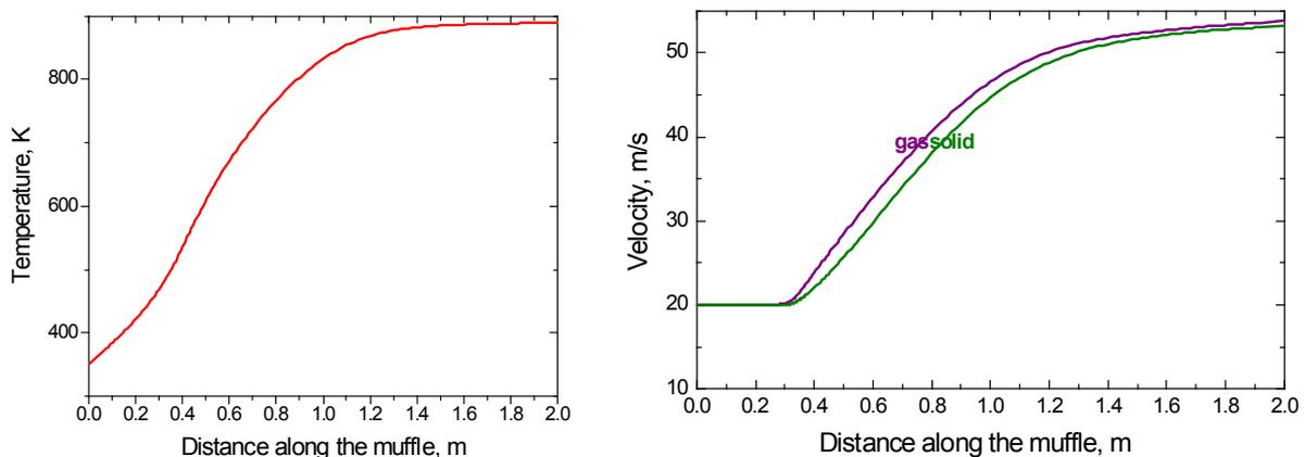
**Figure 5** – Temperature and velocity of the products along the muffle
