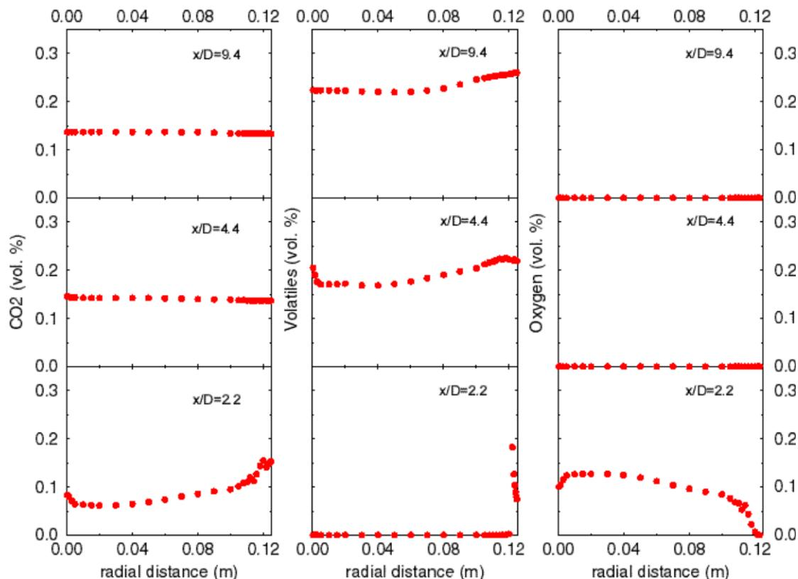
Figure 9 – Predicted radial profiles of carbon dioxide, oxygen and volatiles concentrations.
