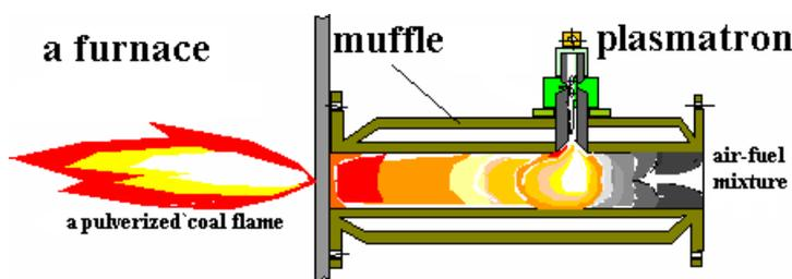
**Figure 1** – Principle scheme of a plasmatron and cylindrical direct flow burner mounting
