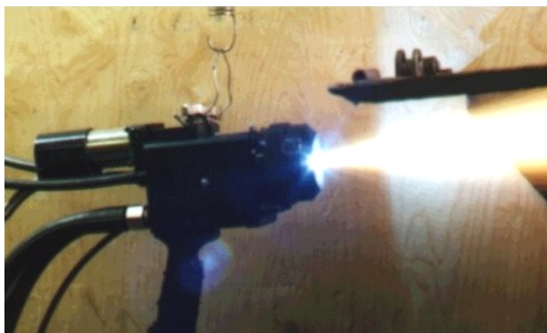
Figure 3 – Spraying with an ADM apparatus.
