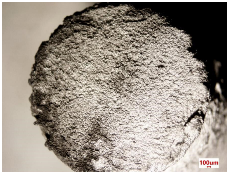
Figure 2 – End surface of a sample made of NZ30K alloy + 0.1 wt.% Ag clad with a layer of silver with copper impurities with a thickness of 1300 nm after corrosion tests in Ringer-Locke solution.
