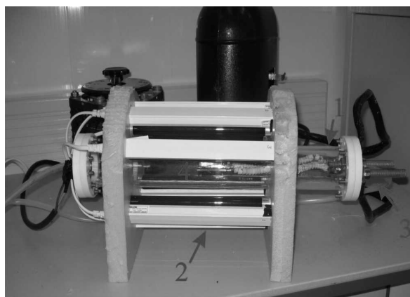
1 – Quartz tube (reaction chamber); 2 – source of ultraviolet irradiation; 3 – clamp terminals, 4– sample holder (substrate holder)
