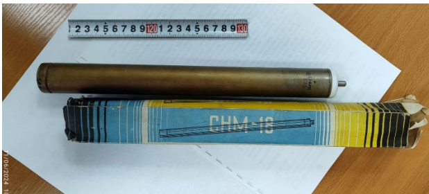
Figure 1 – SNC18 Slow neutron counter tube.
