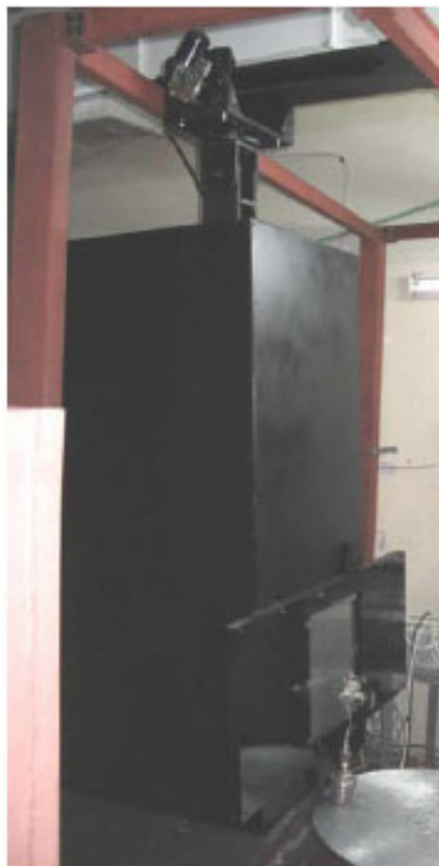
Figure 2 – A view of the detector with scintillators and CCD camera.
