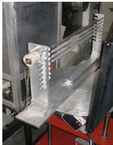
Figure 15 – Holder for nuclear fuel put on the sample holder.
