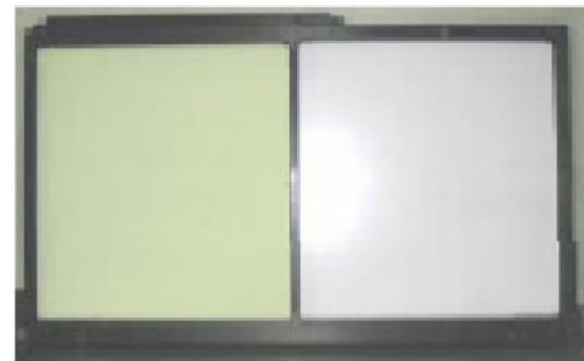
Figure 3 – The scintillator for neutrons (left) and the scintillator for gammas (right).
