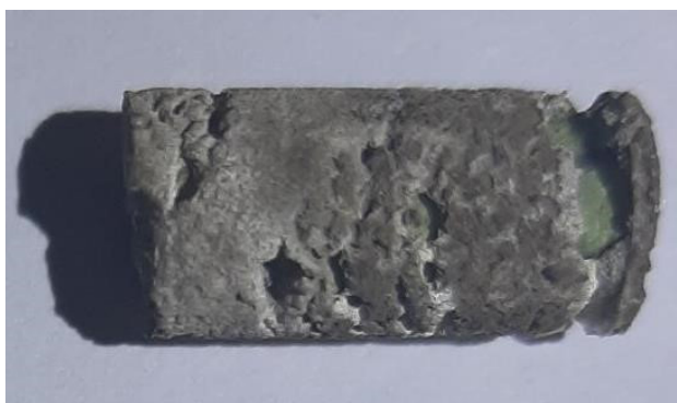
Figure 3 – Cylindrical surface of a sample made of NZ30K alloy + 0.1 wt.% Ag clad with a layer of silver with copper impurities with a thickness of 1300 nm after corrosion tests in Ringer-Locke solution.
